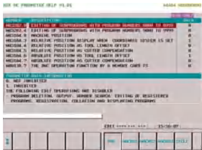
Easy NC parameter help Operator can check some useful parameters for easy operation.
