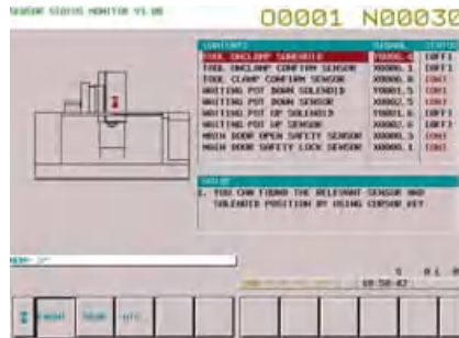
Sensor status monitor Solenoid valve and Sensor status can be checked without the electric diagram.
