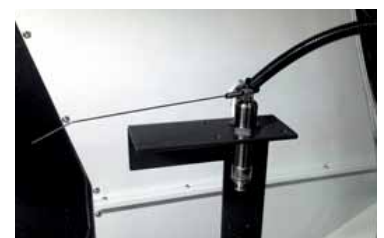
Automatic tool breakage detection
