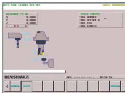
RENISHAW GUI (Tool measure std. ) (Work measure opt. ) Tool & work measure system of Renishaw is operated on conversational screen.
